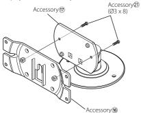
2 Install the display unit to the display bracket (Accessory (6)).
